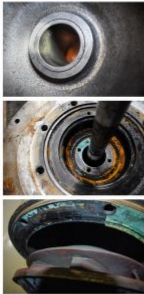
During the commissioning and startup of an alumina processing plant in the Middle East, a significant recurring pump issue was causing delays to the commissioning of the facility. When de-energizing the equipment, the live steam condensate vertical can pumps experienced repeated failures of all installed units. These seizures occurred at both the design fluid temperature and when pumping cold water.
