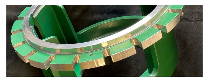
State of the Art Parts: Hydro Parts Solutions recently supplied a new bearing cartridge and adaptor piece for an OH2 pump from a Caribbean rum distillery. The customer had no spares for these components and was in a critical situation because both parts had failed and were unusable.
