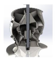
When the experts at Hydro were called on to reverse-engineer parts for a large circulating water pump in the Caribbean, they were concerned to discover an OEM-provided suction bell had failed during service. All internal ribs were lost and the bearing holder was found loose within the assembly. Not only had the suction bell failed, but the customer was facing excessive lead times for the parts needed for the refurbishment of the pump.
