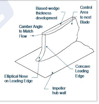
Figure 5 - Biased-wedge impeller
