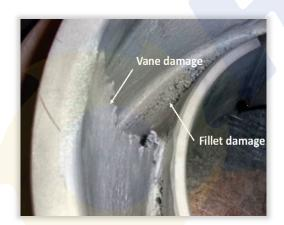
Figure 3 - Impeller damage due to hydraulic instability or suction recirculation Secondly, the hydraulic instability creates a nonhomogeneous fluid-field surrounding the impeller. This results in large radial loads pushing the rotor in different directions and causing contact at closeclearance areas – normally the wear rings. This is analogous to the uncomfortable feeling of flying through clouds.
