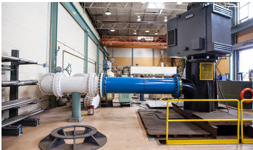
IMAGE 4: The performance test results showed that the subsynchronous bearing whirl vibration was reduced to acceptable amplitude levels.
