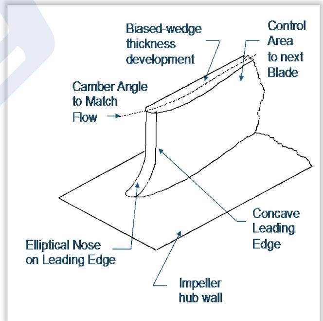
**Figure 5 - Biased-wedge impeller**
