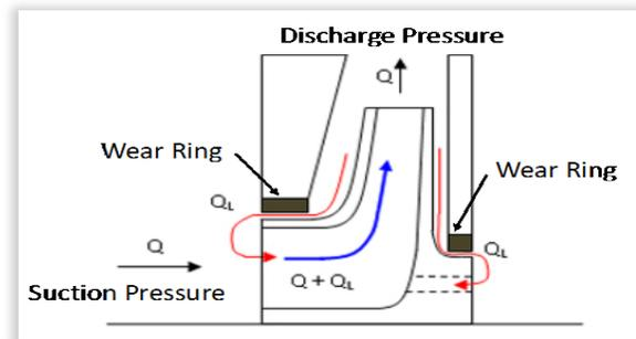
**Figure 4 - Internal recirculation**
