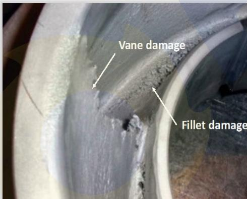
**Figure 3 - Impeller damage due to hydraulic instability or suction recirculation**
