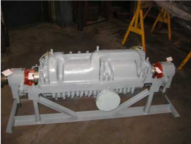
Figure 1. The 9-stage boiler feed water pump
