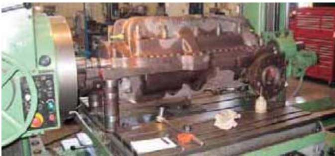
Figure 4. Line boring the pump case
