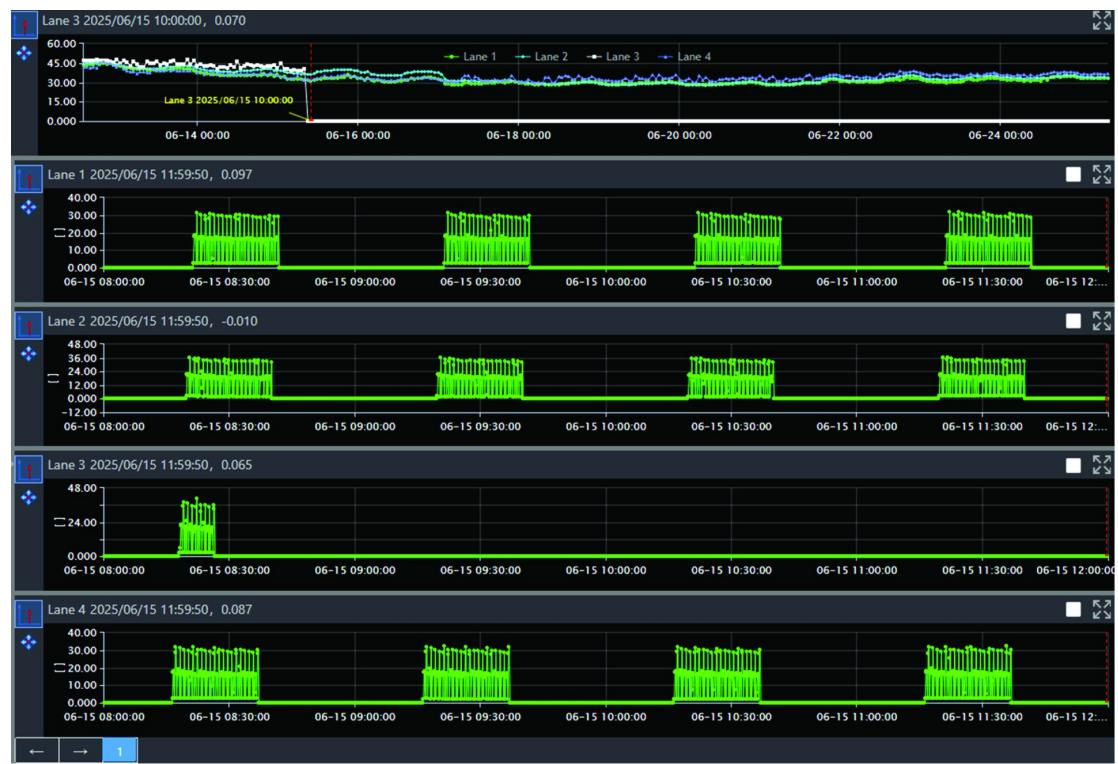
At a midstream pipeline station receiving batches of different refined products, Centaur captured upstream and downstream pressure on three pumps and correlated those signals with vibration. As batches transitioned, operators could see pressure deviations drive vibration change—flagging anomalies early and guiding intervention before conditions escalated. Long-term pressure trends also revealed efficiency drift tied to wear, informing work scheduling when it created the most reliability value.
