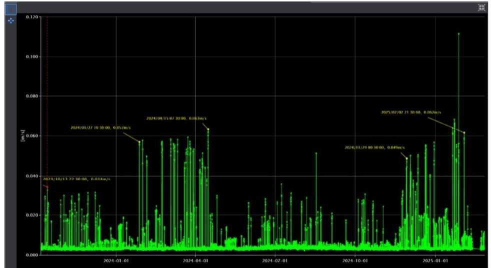
While the system showed no overt performance issues, long-term data revealed that motor vibration amplitudes consistently increased 150–200% during colder months. Frequency analysis identified discrete peaks linked to transient cavitation events and turbulence, particularly on the pump and recirculation line.
