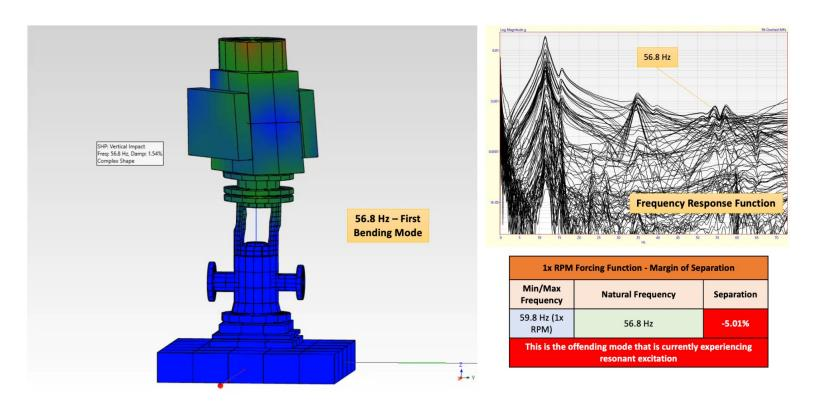
Vertical pumps are especially susceptible to minor conditions that can result in elevated vibration amplitudes. The vertically suspended design and long stationary element lengths often combine into natural frequencies that are near forcing frequencies, such as running speed or even sub-synchronous faults. The complexity of these issues makes it difficult to diagnose and resolve persistent vibration issues with the type of data that is routinely available to the end users.
