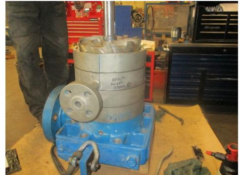
In this case, a small shop had completed several repairs that had resulted in high vibration and performance issues. These pumps were a legacy design that was no longer supported by the OEM and required engineering knowledge to properly refurbish and set the balance device. As such, it was important to find a repair partner that had a strong understanding of pump design. The plant worked with Hydro's Scotford facility to bring these "bad actor" pumps back to optimal performance.
