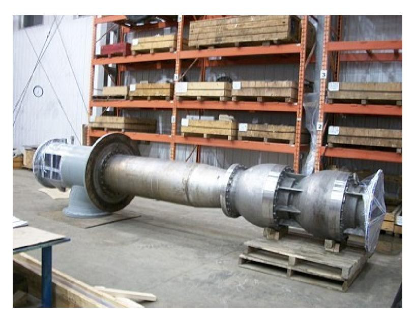
**Application: Pond Process Water** Pump Details: Byron Jackson 32KXL Pump Type: Multi-Stage Vertical
