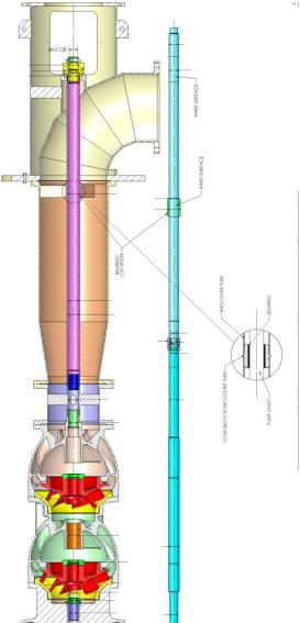
This pump had been "upgraded" by replacing the upper bearing with an enclosure tube, which was not part of the original design. The lack of that bearing contributed to the instability of the top shaft and may have lead to the pump's failure.
