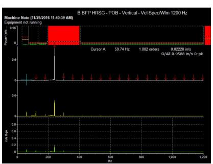
This scenario was experienced by a power utility in the Southeastern US when they ran into significant vibration increases after one of their boiler feed pumps was refurbished by a local repair shop.
