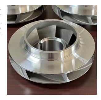
The end user chose to have the new impellers manufactured out of CA6NM using investment casting, which provides a smoother surface finish to slightly increase the impeller efficiency. Hydro Parts Solutions drove the project from casting package design through final machining, with the impellers being cast and finish-machined within 6 weeks.
