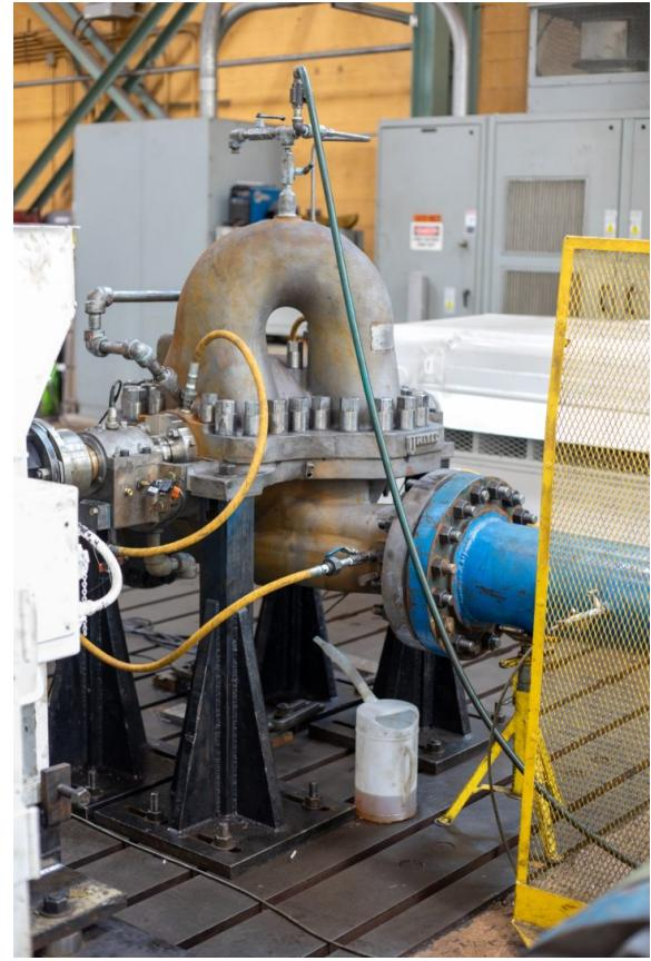
The pump performance specifications were developed by system engineers and communicated to Hydro. The pump's original design condition was modified to provide the necessary differential pressure required for the desired flow rate – for today and in the future. This will be achieved without the use of DRA or with little added to the system.
