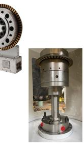
Historically, thrust has been a calculated value based on the impeller design and other pump parameters; this calculation is an approximation and has a margin of error. Axial thrust can be more accurately assessed through testing, but direct measurement of the thrust across the profile of a pump performance curve is not typically performed by OEMs.
