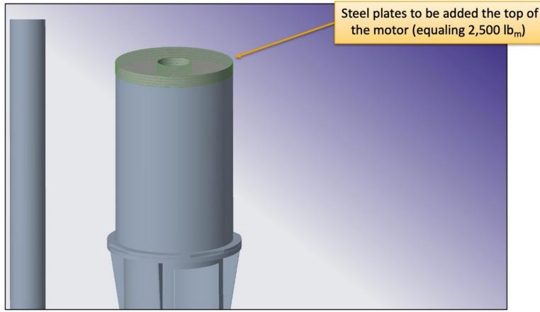
The proposed change was implemented in the field and the plant saw an immediate reduction in vibration from 0.47 IPS 0-P to 0.1 IPS 0-P. Using in-field testing and advanced analytics supported by modeling software allowed the site to not only troubleshoot the problem, but execute a solution that solved it on the first try.
