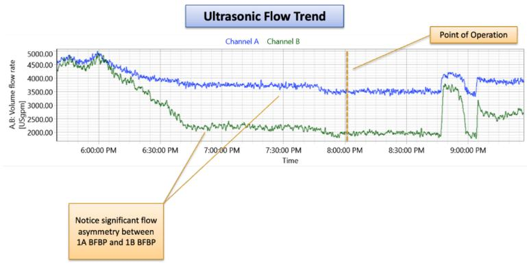
Testing of the boiler feed pumps revealed elevated amplitudes near 300MW and an axial structural resonance on the drive end of the 1A pump. The 1B pump also had a structural resonance excited by vane pass on the inboard bearing housing. It was recommended that an experimental modal analysis (EMA) be completed on both pumps to determine the best actions to resolve the resonance issues.
