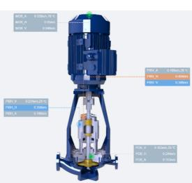
Here's an example of the process at work. In this case, a machine train's vibration amplitudes trigger an alarm:
