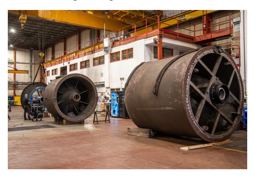
A nuclear utility had a large circulating water pump with severe vibration issues that required refurbishment in an emergency time frame. <u>Hydro's Aston, PA service center</u>, which has a 50-ton crane and a history of providing quality repair for nuclear non-safety related equipment, was chosen for this work. Despite the unique challenges in machining and maneuverability presented by large pumps, the
