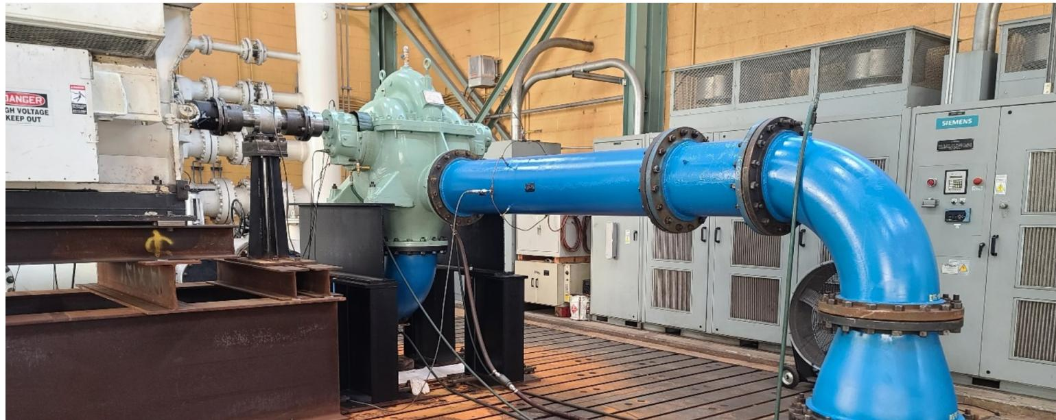
A municipal water treatment plant recently had one of their service water pumps refurbished. The refurbished pump is a single-stage, bottom suction BB1 (between bearing) pump with a double suction impeller. In order to validate the performance of the pump, the plant requested testing services from the Hydro Performance Test Lab. The testing services included a Hydraulic Institute certified performance test, a Net Positive Suction Head (NPSH) test, and a bearing housing vibration test.
