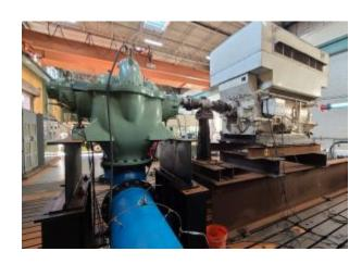
The bottom suction design of the pump provided some challenges in the design of the test layout and in conducting the NPSH test. The bottom suction design of the pump did not allow for the typical piping layout design. Instead, the mounting feet of the pump needed to be elevated and supported at least 5 feet from the floor to correctly connect to the suction manifold. Changing the pump mounting elevation meant that the motor also needed to be elevated and supported at the same height.
