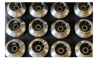
State of the Art Parts: Hydro Parts Solutions recently supplied a new impeller as part of a project to improve the operation of a pump that was not performing per the OEM curve. The first step in the process was reverse-engineering the used sample impellers. The reverse-engineered model was used by Hydro's Global Engineering team to perform a computational fluid dynamics (CFD) analysis to determine the best possible hydraulic design for the plant's expected operating range.
