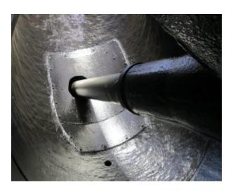
Following the installation of all the plates and gussets, the entire internal section of the elbow was coated to protect and improve the water flow. The pump was returned to the customer in early February 2013 and remains in operation today.
