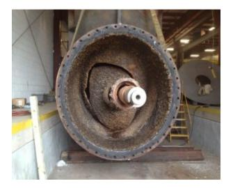
A critical vertical pump for a 750 MW unit was sent to <u>Hydro South</u> in mid-December 2012 for inspection and repair. The massive pump weighed more than 66,000 lbs. and was 32 feet long and 12 feet tall. When the pump was disassembled, Hydro South's engineers discovered that a large 42" x 68" section of the discharge elbow was broken, allowing direct flow to bypass the turning section and flow directly into the stuffing box area.
