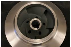
With the critical timeframe in mind, the Hydro Parts Solutions team dedicated its resources to this project. They were able to reverse engineer the part, verify the model, design the mold, cast the component, and provide final machining within a 3-week time frame. The refurbished pump was delivered to the plant before the backup unit degraded further, avoiding costly downtime.
