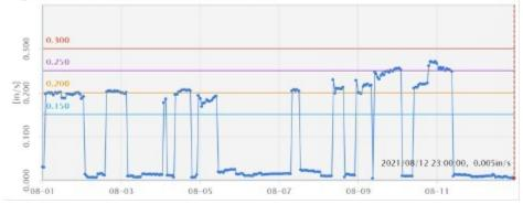
The monitored data identified a dominant excitation frequency at 1x run speed (29.688Hz) with harmonics. The team at Hydro's Monitoring & Diagnostic Center suspected that misalignment may be the root cause of the elevated vibration amplitude readings.
