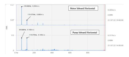
Phase analysis has been performed on the pump inboard and motor inboard sensor locations to allow Hydro's engineers to further confirm the diagnosis of misalignment. Misalignment is characterized by a phase difference of 180° ±30° between the coupled components. Referencing the phase difference between the
