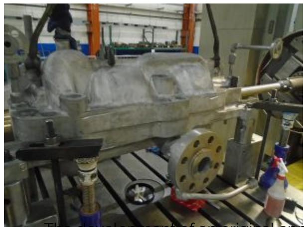
Hydro performed a final cleaning and passivation check to ensure that no iron contaminants were found in the newly repaired casing. With negative results on the passivation check, Hydro was able to ship the casing back to Europe (Figure 4). The customer was impressed with the innovative approach and with the management of the many details in this unique project scope. The creative approach saved the nuclear plant time and money, while also reducing their risk.
