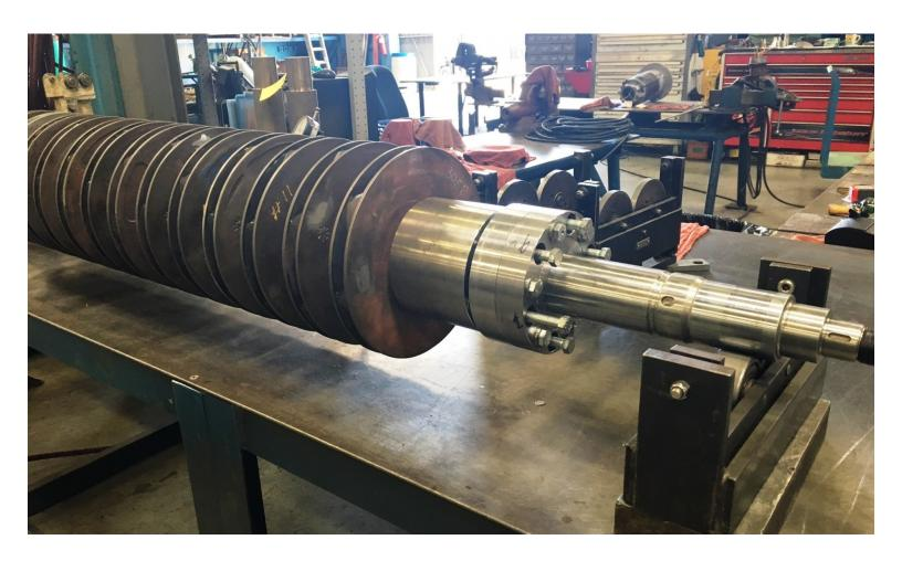
A major power plant in the United States experienced high vibration and recirculation issues with several ring section (BB4) boiler feed pumps, resulting in multiple catastrophic failures and unplanned outages. This case study details one of the pumps that was shipped to an aftermarket pump service center for a full analysis, troubleshooting, repair plan, rebuild and performance testing.
