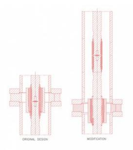
The double row deep groove ball bearing that was chosen to replace the angular contact bearing is able to handle axial loads in either direction and will not be at risk of unseating due to axial upthrust. This bearing design will also protect the mechanical seal by restricting rotor axial movement in both directions. In order to accommodate the new bearing, the bearing housing was modified.
