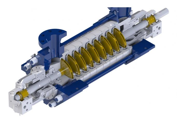
The pump shaft is the central component of the rotating element and is responsible for transmitting energy to the rotating components. The shaft carries the impellers, sleeves and couplings for the rotating element assembly. The stiffness of the combined assembly is responsible for ensuring that the pump stationary components do not come into contact with the rotating components.
