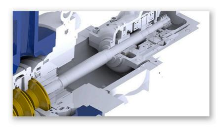
Many high-energy multistage machines use thrust compensation devices to limit the amount of axial thrust a bearing must accommodate.
