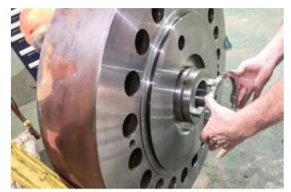
The combination of the discharge head extension that protrudes into the casing, the shim compensator set, and the internal assembly determines the crush on the internal suction gasket. The insufficient thickness of the compensator shims resulted in an unloaded gasket, preventing the formation of an effective seal. The failure of this gasket allowed internal leakage from the high pressure discharge chamber back to suction.
