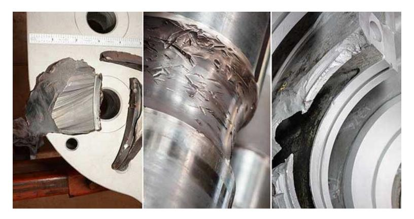
Efficiency and reliability are at the forefront of a successful pumping system. As such, unplanned outages can be a detrimental disturbance to the overall operation. In this case, the end user's high pressure multistage BB5 barrel pump was experiencing severe vibration, unstable performance, and failure in the field leading to unit shutdown.
