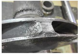
A major steel plant on the East Coast had been experiencing catastrophic failures with its five-stage descaling pumps. The plant operated using three multistage axially split (BB3) pumps with two spares. All five of the pumps had a mean time between repair (MTBR) of two years. In this case, the plant water quality was considered to be less than ideal, and the entrained abrasives were a factor contributing to the repeated failures.
