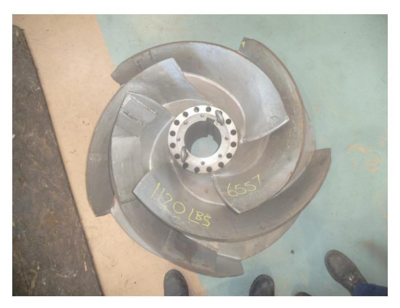
Vibration issues with a two-stage pump forced a major steel manufacturer to remove the pump from service. Due to incorrect weights welded on an impeller, a steel manufacturer called upon Hydro to repair and balance a two-stage pump.
