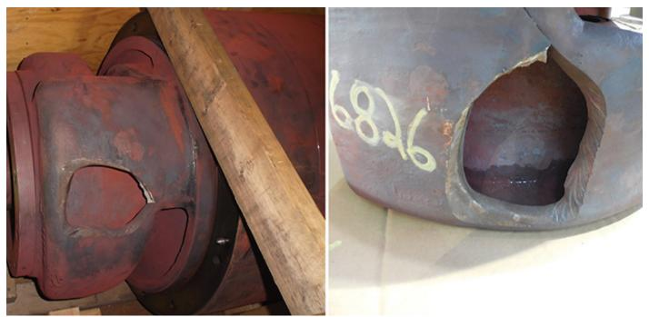
The first-stage twin volute is a complicated casting, which failed during operation as a result of poor design.
