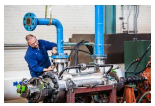
A Western European nuclear power plant was having difficulty meeting the necessary hydraulic performance at runout for two centrifugal charging pumps. The system needed 30 ft of Net Positive Suction Head required (NPSHr).
