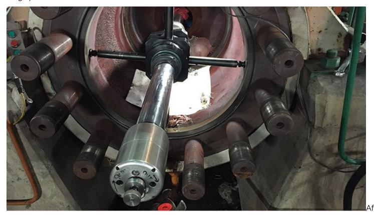
rebuilding a cartridge and returning all operating clearances to specification, the good work can be greatly affected by installing the cartridge into a distorted barrel and/or discharge head combination.
