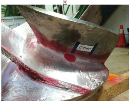
Other shortcuts had been taken during pump manufacturing. A machining concentricity error was found between the suction bearing and liner during the course of a mechanical setup check. This caused damage to the impeller and liner that included heavy eccentric wear in the suction bearing. A concentricity check of the complete column assembly was performed on-site.
