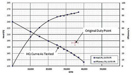
Over time, the design of the impellers also drifted away from optimal because no testing or verification of the performance took place. Cavitation and insufficient service water continued until the pumping station could not keep up with plant demand. As Figure 3 shows, field pump assessments and
