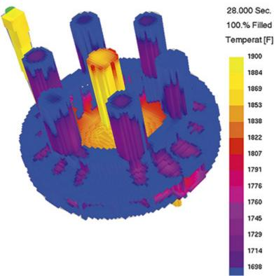
Once the geometry is defined, performing material solidification simulation of the casting is critical. The solidification software is designed around computational fluid dynamics, which allows engineers to simulate the velocities and temperature gradients of the metal throughout the pour cycle.
