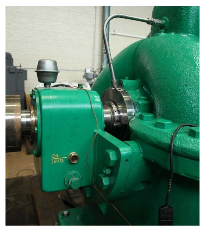
Once the engineering review was complete and all the modifications were agreed upon, Hydro went to work. The shaft was modified to a stepped design and the distance between the bearings was shortened to reduce deflection at the seal faces. The sleeve bearings were removed and ball bearings were put in to greatly handle the axial thrust of the rotor, thus stabilizing the shaft and lowering vibration. New mechanical seals were installed along with newly manufactured bearing housings,
