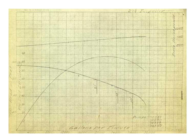
The rotating equipment engineers at the refinery wanted to better understand the operating characteristics of these pumps, which were originally built by Cameron in 1928. Because these pumps were installed so long ago, there was no NPSH data available and the pumps' best efficiency point was not known.
