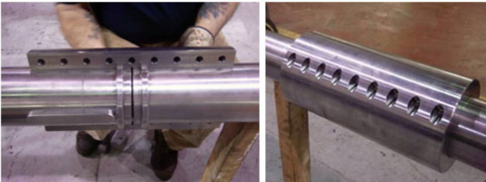
New shafts and shaft coupling components during and after assembly
