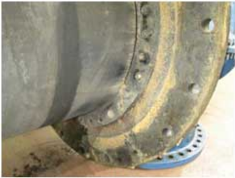
Column pipe upper flange as-received
