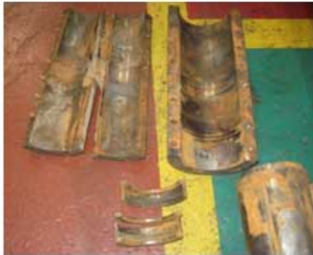
Destroyed shaft coupling and hardware
