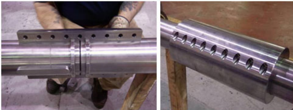
New shafts and shaft coupling components during and after assembly
