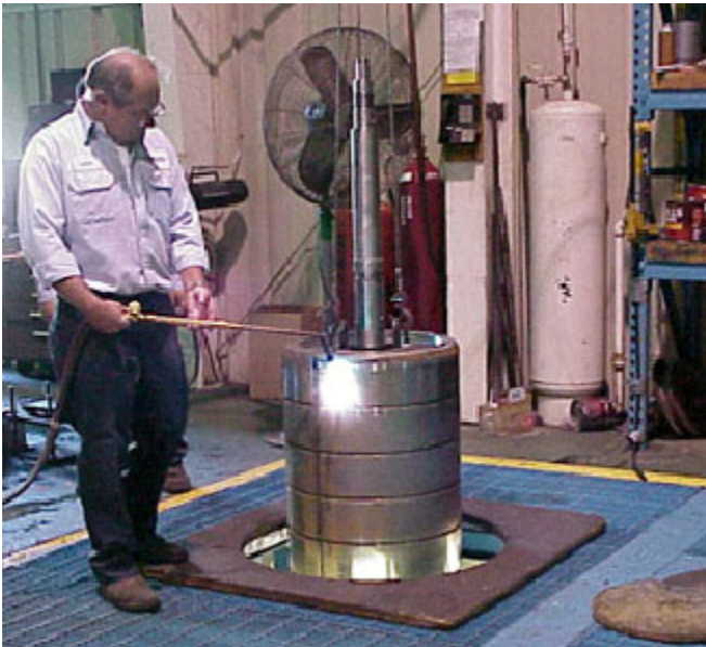
Figure 2. Vertical assembly of a multistage barrel pump
