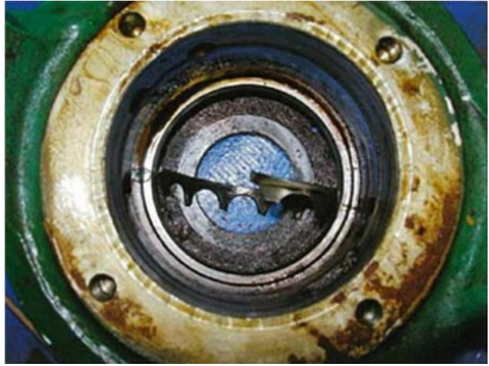
(Left) BFP Installation (Right) Bearing Cage from a previous repair
