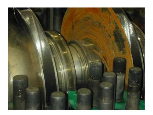
Excessive wear was noted at all running clearances. Discussions with the plant subsequently revealed
