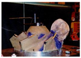
The service center's hydraulic design engineers analyzed the performance requirements of the original design using CFD (computational fluid design) and data that was available from the existing impeller to recreate the impeller's hydraulic profile. A CAD drawing was developed and electronically transferred to the foundry for the mold used to cast the impeller vanes.
