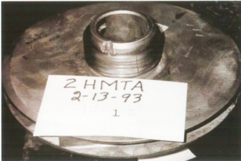
Figure 2. Broken impeller wear ring due to improper hardness (i.e. too high for tension)
