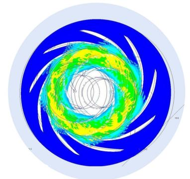
After field data is taken and areas of inefficiency and improvement are identified, analytical software is critical in understanding how to make changes that will improve system performance. Computational fluid dynamics (CFD) allows custom hydraulics to be designed. It also predicts fluid behavior when modifications are made that might influence pump performance, such as changes in the intake of the
